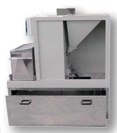
This machine has been designed to save time normally required to separate tumbled pieces from abrasive elements of any type, shape and size.
